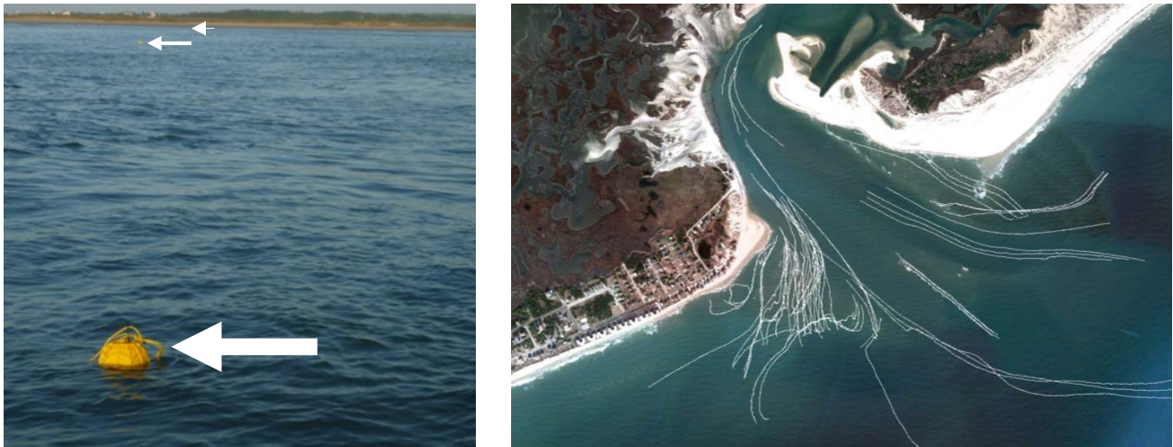
Figure 2. Left Panel: A portion of the miniature wave array deployed to drift across shoals. Right Panel: 10Hz (x,y,z) inertial and GPS data sampling from miniature wave buoy array.
