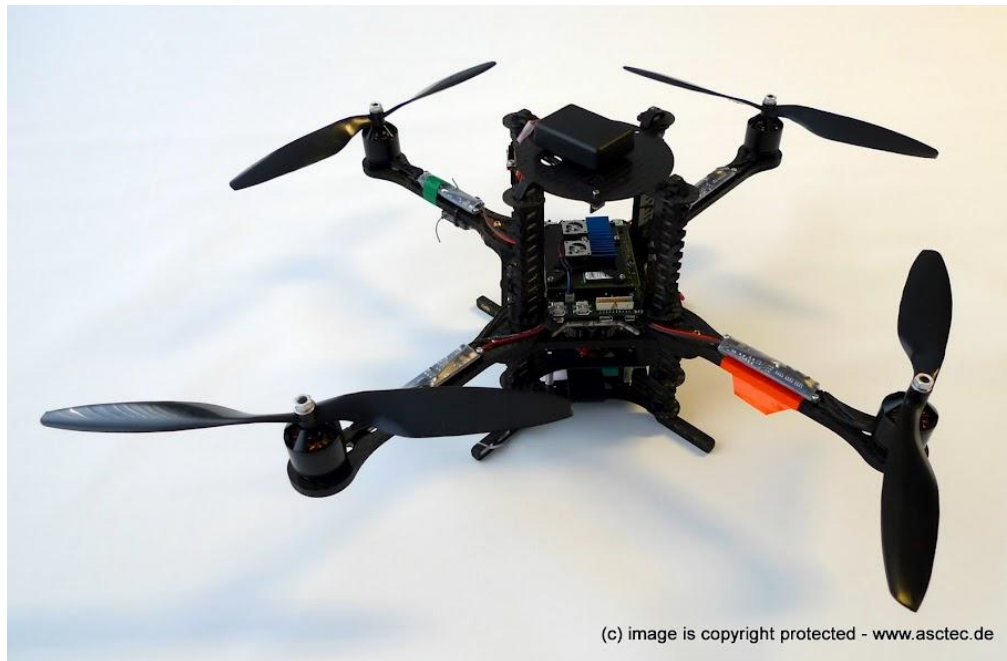
Figure 2-5: The Ascending Technologies Pelican in its standard configuration. The orange tape is used to denote the front on the vehicle. (photo source: Ascending Technologies GmbH)
