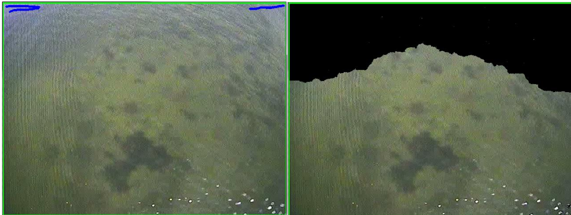
Figure 3-8: GrabCut algorithm applied to an aerial image of the algal bloom. The only user input provided came from defining the pixels under the blue lines as belonging to the background.
