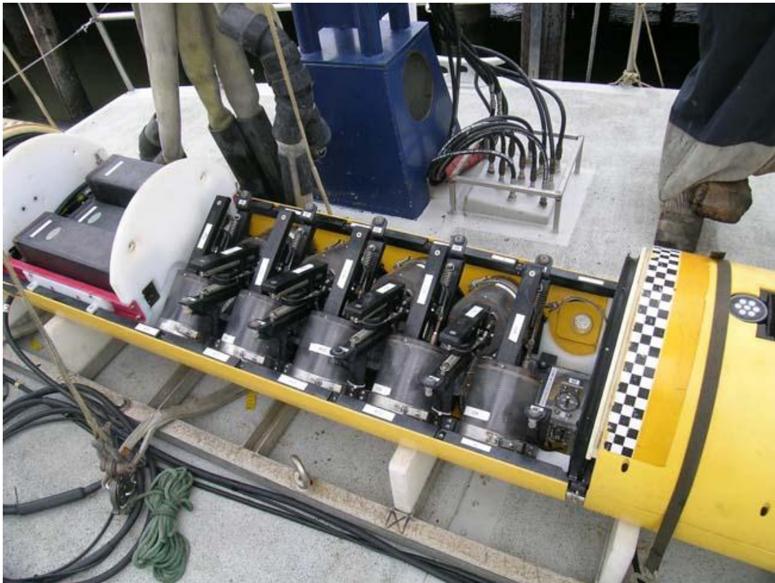
Figure 1-5: The GULPER water sampling system shown mounted in the midsection of a 21" diameter AUV. (photo credit: MBARI)
