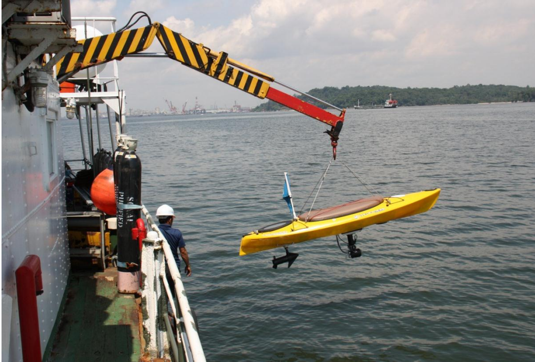
Figure 1-4: A SCOUT equipped with a pan/tilt mounted ADCP being deployed from MV Mata Ikan on the Johor Strait, Singapore.
