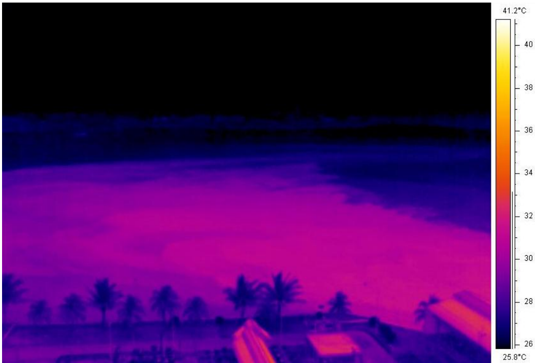
Figure 1-7: A thermal image of the Senoko power station cooling exhaust. While a camera could be mounted on a high smokestack here, the low angle of incidence affects the accuracy of temperature readings. In other locations vantage points such as this one are simply not available. (image source: Tawfiq Taher)
