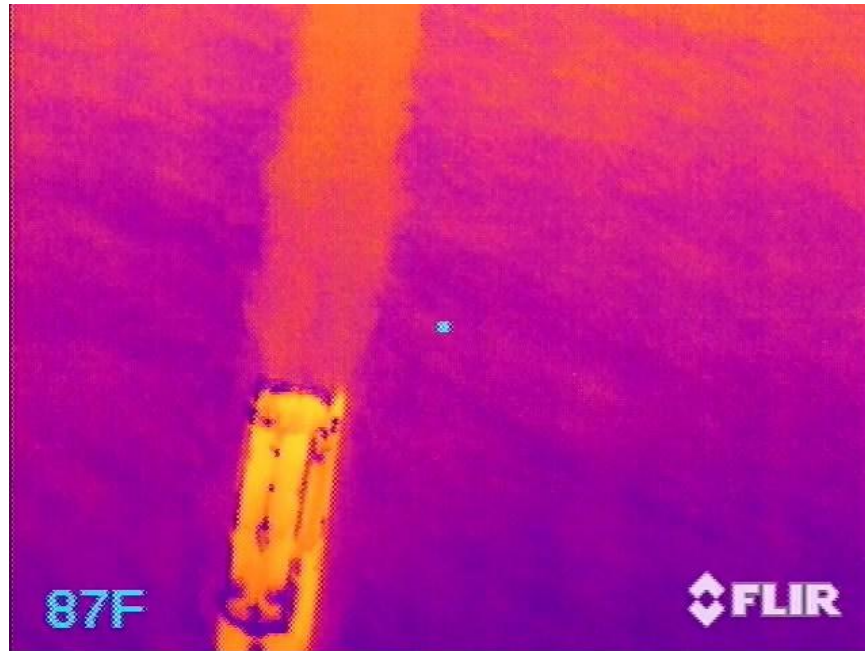
Figure 2-2: Frame capture from the Tau 320's analog video feed showing a boat and the warm water in its wake as it passes underneath the quadrotor.
