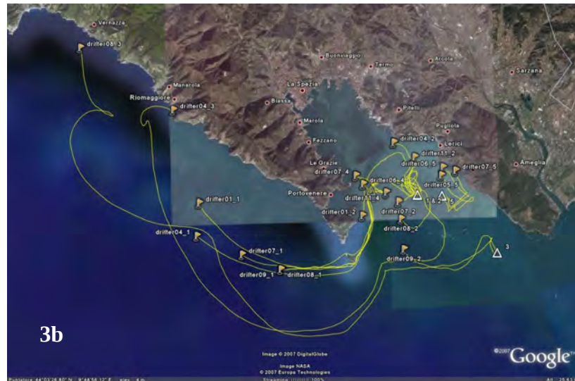
Figure 3: a) trajectories of a cluster of 5 drifters launched in the Ligurian Sea; b) trajectories of 5 clusters of drifters launched in the Gulf of La Spezia during the period June 16-28 2007. The white (orange) triangles indicate launching (ending) points. Courtesy of P.Poulain (OGS)
