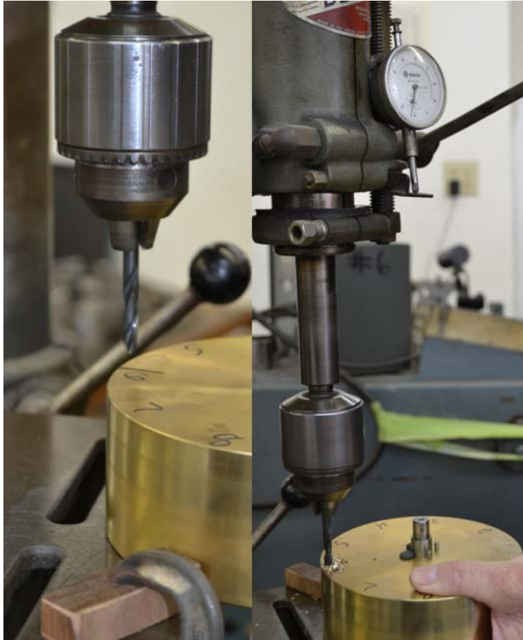
Figure 68. Image of the wheel being drilled
