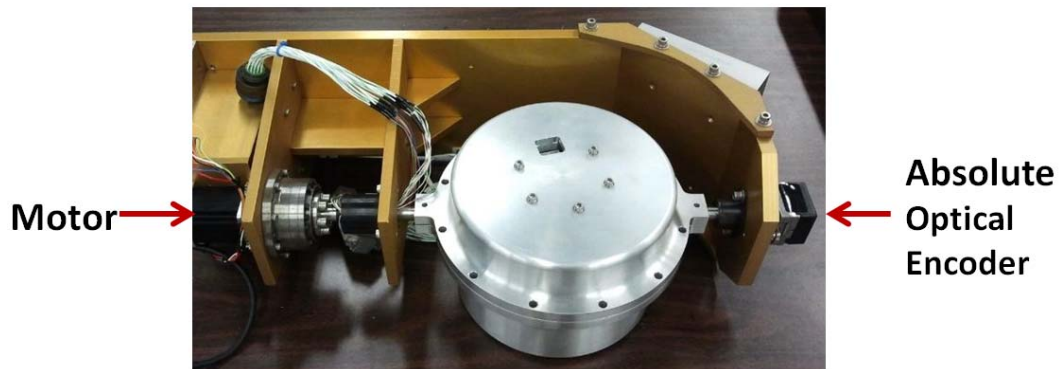
Figure 70. Gimbal and momentum wheel assembly integration
