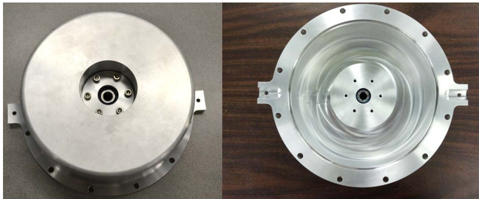
Figure 61. Bearing side case and duplex bearing integration
