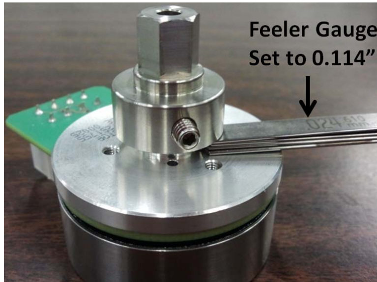
Figure 59. Motor connector positioning
