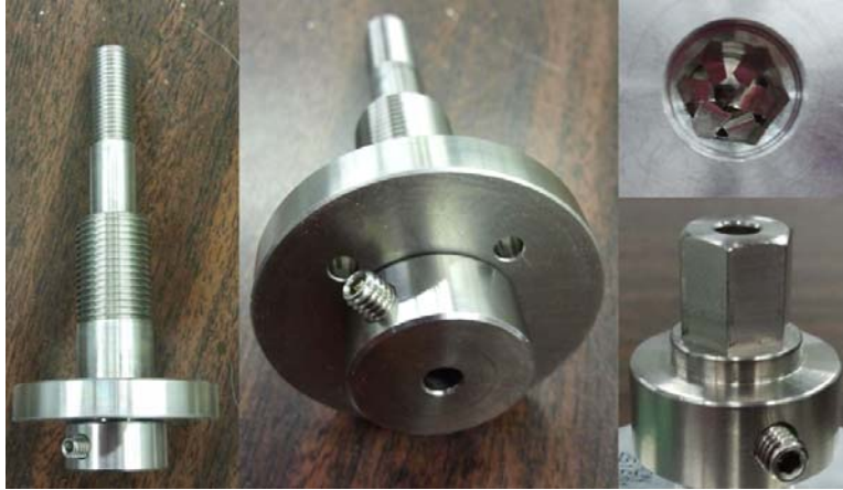
Figure 51. Shaft and motor connector integration
