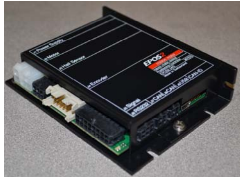
Figure 72. Maxon EPOS 24/5 position/velocity controller
