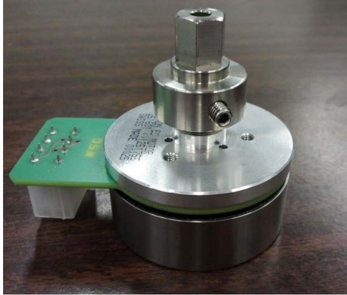
Figure 57. Motor and motor connector integration
