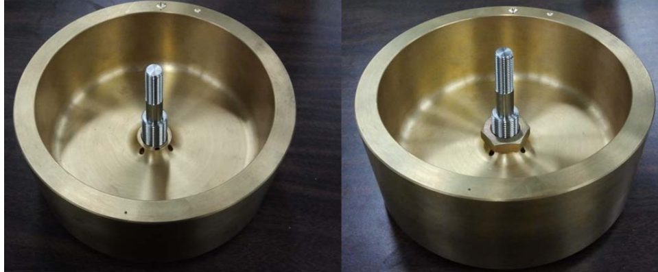
Figure 49. Momentum wheel and shaft integration
