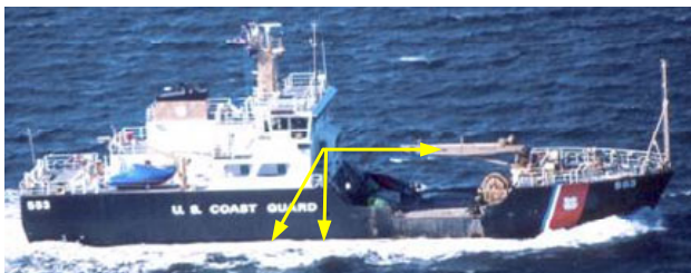
Figure 12 – IMU axis orientation on a vessel.
