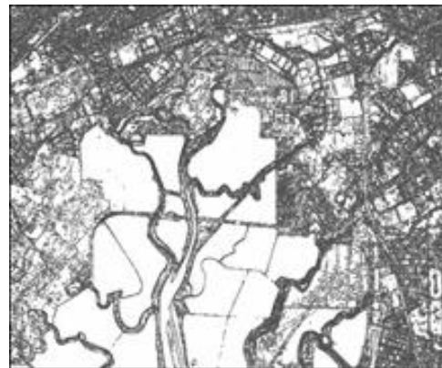
Figure 4d: Spectral Texture Method ASM texture feature for simulated MSI image cube.
