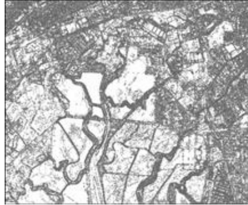
Figure 9b: Spectral Texture Method Mean texture feature for the HSI image cube.
