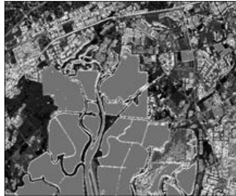
Figure 6d: Spectral Texture Method Correlation texture feature for the simulated MSI image cube.
