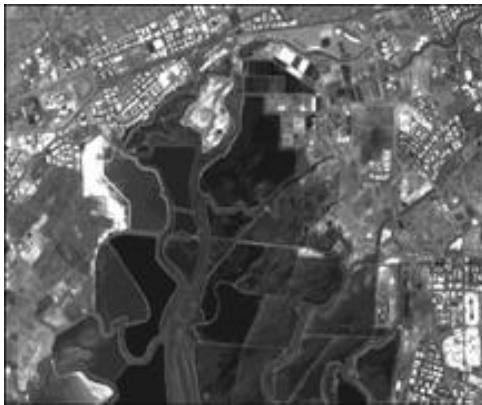
Figure 8c: Haralick Method Variance texture feature for the simulated MSI image cube.
