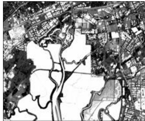
Figure 8d: Spectral Texture Method Variance texture feature for the simulated MSI image cube.
