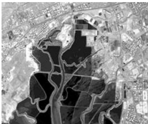
Figure 2a: Haralick Method Quantization image created for the HSI image. All 224 HSI bands were summed to simulate a panchromatic image.
