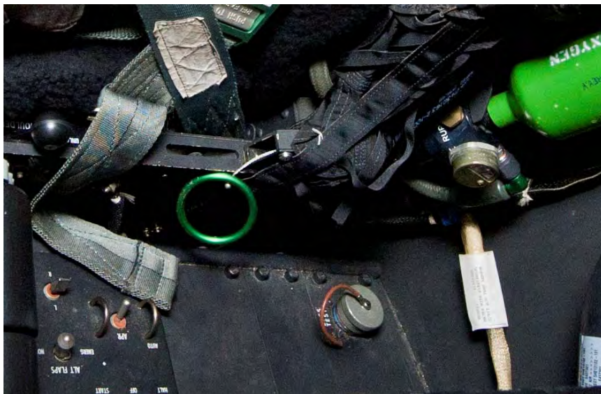
Figure 16- Manual EOS activation ring fallen below lip of seat. (Tab CC-5 and Tab Z-8)
