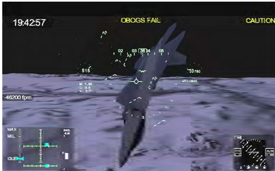
Figure 6 19:42:57 – MA parameters during MA 240 degree roll to the right resulting from stick and pedal inputs. (Tab EE)
