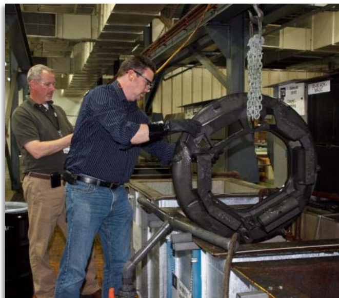
M1 Copula during SurTec 580 process
