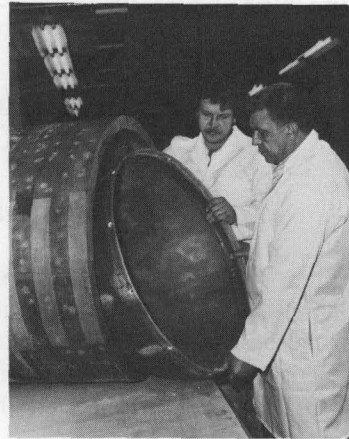
Craftsmen Removing a Fiberglass Lamination from a Mold in the Plastics Shop
