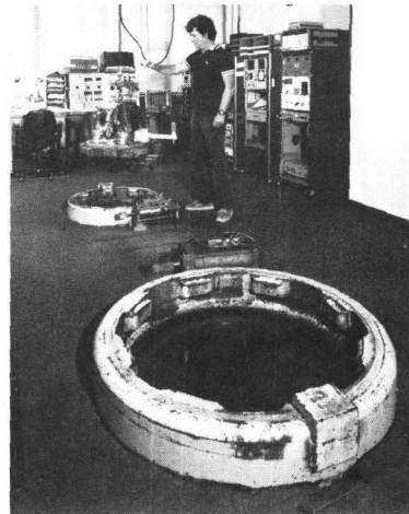
Technician lowering the cover to the smaller of the two ports of entry/exit to the anechoic tank pressure vessel in preparation for a test. The tank is used to test various types of sonar transducers as a function of temperature and pressure.
