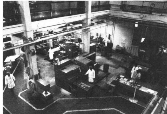
Mills, lathe, and matching center shown here are run by punched paper tape or by manually inputting computerized data
