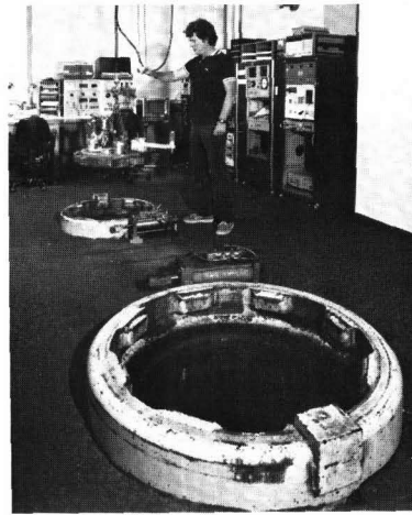
Technician lowering the cover to the smaller of the two ports of entry/exit to the anechoic tank pressure vessel in preparation for a test. The tank is used to test various types of sonar transducers as a function of temperature and pressure.
