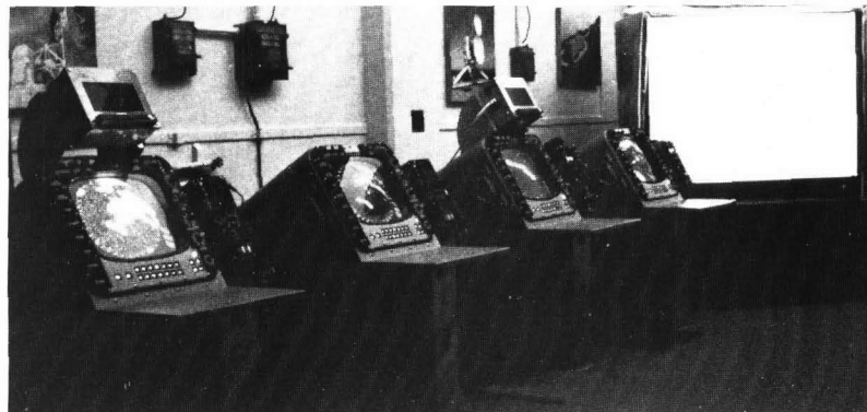
Radar display and distribution systems experimental facility at the NRL Chesapeake Bay Detachment (Chesapeake, MD) showing four SPA-25G microcomputer-driven, raster radar displays and a projection TV display monitor
