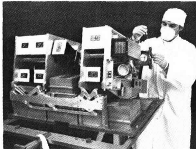
The Remote Atmospheric and Ionospheric Detection System (RAIDS) is an array of eight optical instruments including imaging spectrographs, spectrometers, and photometers that will measure ionospheric and thermospheric airglow emissions at wavelengths from 50 to 870 nm over the altitude range 75 to 750 km on the earth's limb. RAIDS, which is a proof-of-concept for future ionospheric weather sensors, will fly aboard the NOAA J weather satellite.
