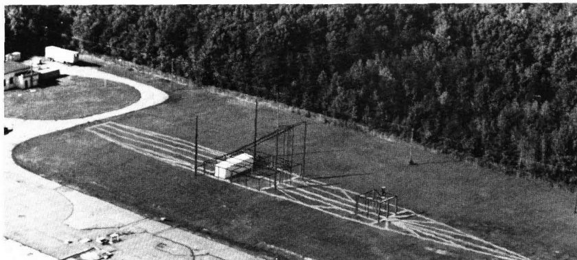
Simulated topside of ship for antenna and communication system measurements at Pomonkey, Maryland, Test Range
