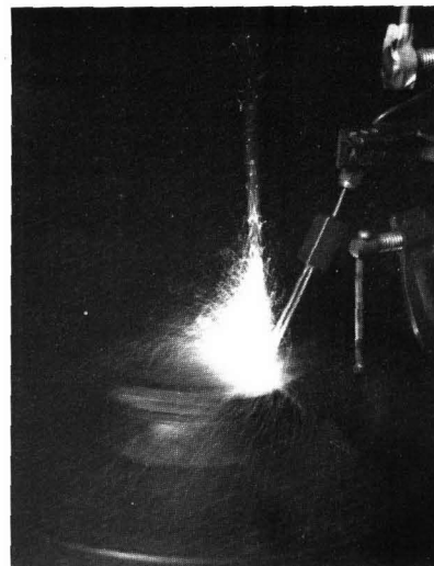
Laser melt particle injection process
