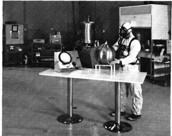
A specially designed and constructed facility for the safe handling and testing of propellants used in Naval Center for Space Technology spacecraft
