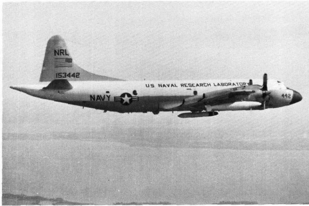
The Tactical Electronic Warfare Division extensively uses a P-3 aircraft as a flying Electronic Warfare Research, Development, Test, and Evaluation Laboratory
