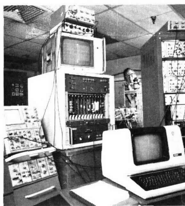
The Focal Plane Array Evaluation Facility consists of the optical sources and electronics required to evaluate monolithic or hybrid infrared focal plane arrays that use charge-coupled device, charge-injection device, direct-readout, or charge-imaging matrix technologies.
