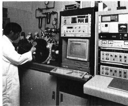
System for plating metallic materials onto graphite fibers or substrates
