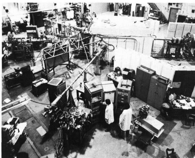
An elevated view showing the NRL 3 MeV Tandem Van de Graaff Accelerator and associated beam lines
