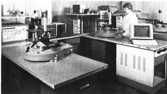
Automated NRL arch measurement of radar-absorbing materials
