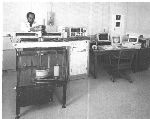
Ultrasonic imaging and analysis system for nondestructive inspection of irregular objects and simple bodies of revolution. The computer-interactive automated system provides acoustic images of bodies fabricated from metals or composites in real time, with visual indicators of defects that may be present.
