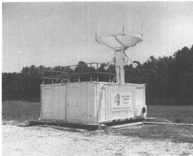
The transportable ground station for the low-power atmospheric compensation experiment (LACE) spacecraft is shown in an operationally ready configuration. Housed in strong, low cost cargo "containers," the station is easily handled for shipment by truck, rail, ship, or aircraft.
