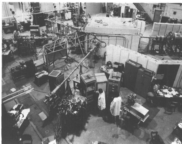
An elevated view showing the NRL 3 MeV Tandem Van de Graaff Accelerator and associated beam lines
