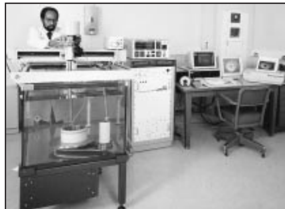
Ultrasonic imaging and analysis system for nondestructive inspection of irregular objects and simple bodies of revolution. The computer-interactive automated system provides acoustic images of bodies fabricated from metals or composites in real time, with visual indicators of defects that may be present.
