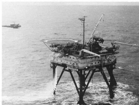
The German Forschungs Platform NORDSEE is used for oceanic and atmospheric surface truth measurements in joint (US/GE/NATO) radar/radiometry/acoustics experiments providing data over a wide range of dynamic conditions
