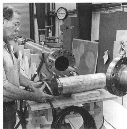
Technician loading sonar material sample for evaluation in Shock-Tube Facility
