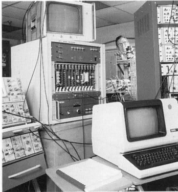
The Missile Seeker Evaluation Facility is a computerized facility that is used to evaluate optical countermeasures to infrared missile seekers and infrared imaging sensors
