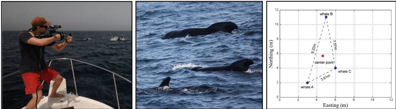
Figure 2: The current stereo geocoding system for 3D localization of whales and quantification of social group cohesion. Left: Photo of the stereo camera system used in August 2012 field cruise, sampling at 4 Hz. Center: Image of 3 pilot whales similar to what is captured by one of the two cameras. Images from both cameras are analysed to find a distance to different whales using the known aperture and calibration values, and then combined with the GPS position and pointing vector of the camera to calculate georeferenced positions. Right: Conceptual illustration of geocoded position estimates of the three animals shown on image in the center. An initial RMS measure of social group cohesion could be derived as the root-mean-squared distance from each whale (dorsal fin location shown in blue circles) to the mean group position (red circle), for a mean group spread of 4.05 m in this example, and with individual distances between animals noted on figure. Range resolution for the current system is better than \pm 1\text{m} at 50 meters distance.
