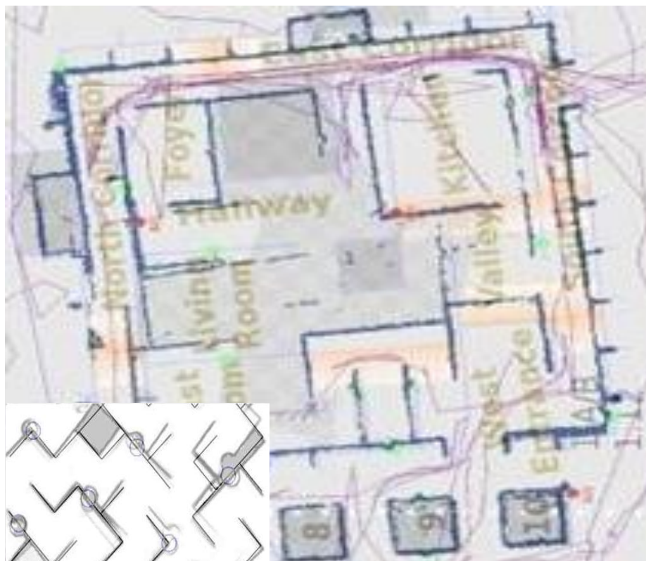
Figure 6: The observed internal structure of the maze in Phase I. The true locations of the barrels are depicted by light green dots; their locations (as determined by the robots) are visible as 'bumps' in the observed data; and the locations of three static OOI are shown as red dots. The mauve lines show the paths taken by the robots. The higher resolution image (inset lower left) shows the effectiveness of the fiducial 'barrel-referencing' technique more clearly.
