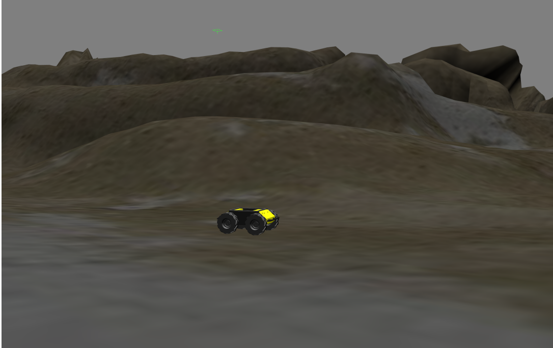
Figure 5.1: Screen shot of a simulated Husky robot in realistic surf zone terrain from the Hector Gazebo package. A very large degree of freedom exist in the specific topography, features and platform that can be combined.
