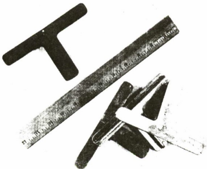
Fig. 2 - Tee-rough castings and the machined surface
