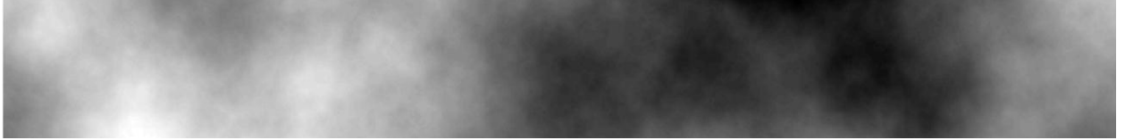
Fig. 3. Gray scale representation of phase screen corresponding to Tatarskii power spectrum with the outer scale L_0 that is seven fold longer than the phase screen width. The phase screen is generated using numerical grid with 8*512 \times 512 ( J=8 ) pixels.
