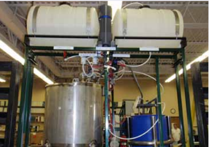
The portable MDH system was designed to treat explosive-contaminated range scrap in the field. The treated metal can be sold as scrap, diverting hazardous waste into a potential revenue stream.
