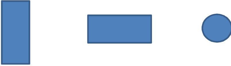
Figure 7: Top View, Front View, and Side View of cylindrical object that from ground could be perceived as spherical in shape
