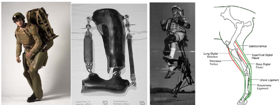
Figure 12: [a] Powered Exoskeleton, [b] Powered Exotendon, [c] Unpowered Exoskeleton & [d] Horse Tendon
