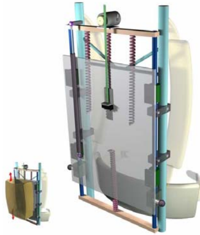
Figure 13: Generator Backpack. From 'Science' (vol 309, p 1726)
