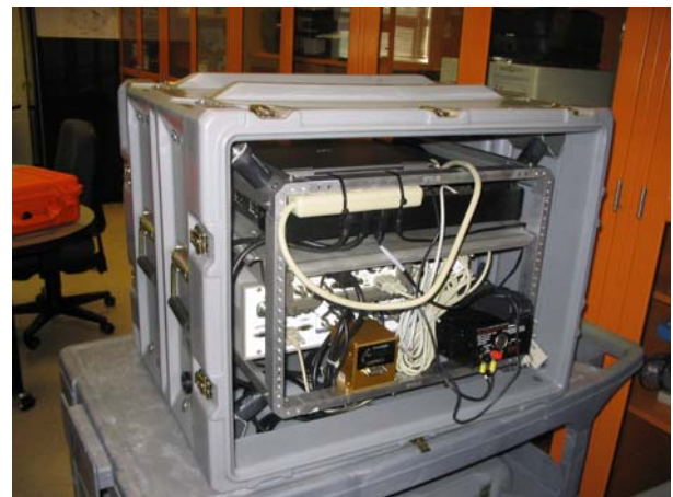
Figure 8 – ASF measurement system, back showing IMU.
