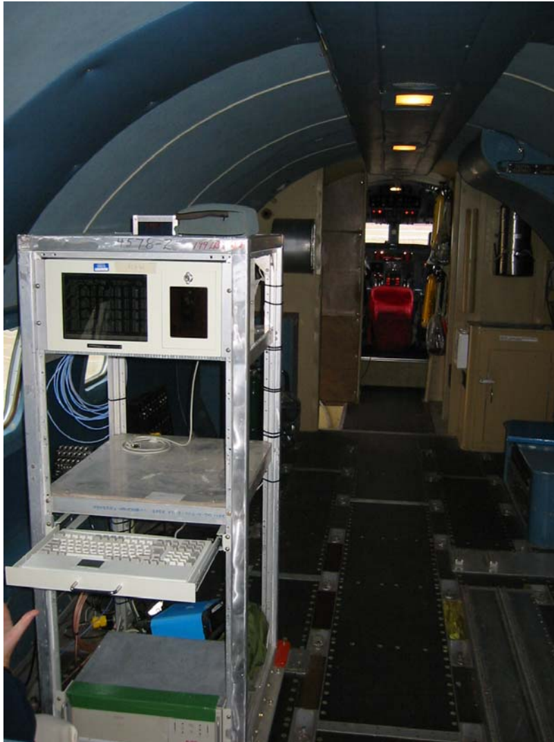
Figure 2: Interior of Convair looking forward; CGA DDC receiver in rack.
