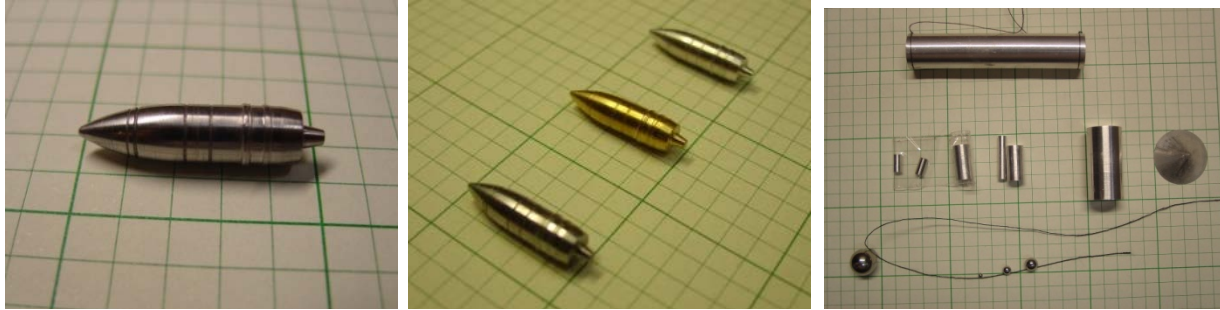
Figure 8. Scaled UXO (left and center) target and canonical target shapes (right) used in tank data collection. Targets are displayed against graph paper with 1in bolded squares.
