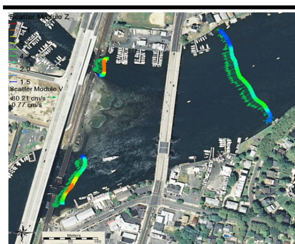
Figure 7. Measured depth-averaged current velocities along surveyed cross sections (CS).
