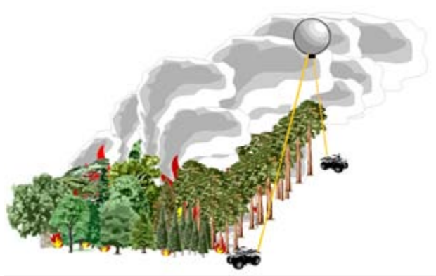
Figure 11. Sampling design to be used by the US EPA aerostat.
