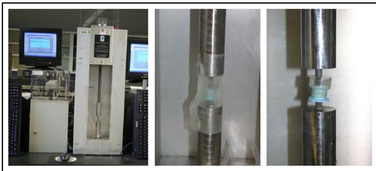
Figure 50. Hydrogen Re-Embrittlement Test Equipment
