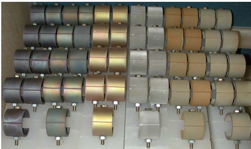
Figure 70. Army C-ring Specimens in the Salt Spray Cabinet
