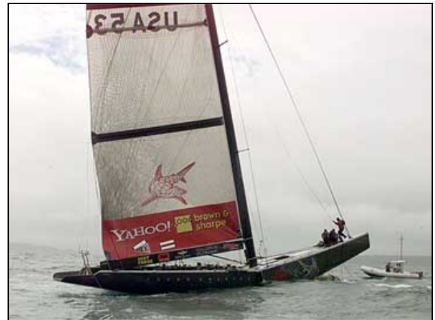
Figure 2: “Young America” suffering deck failure during the 2000 America’s Cup
