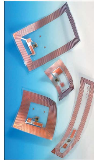
Figure 3 - Passive TI RFIDs
