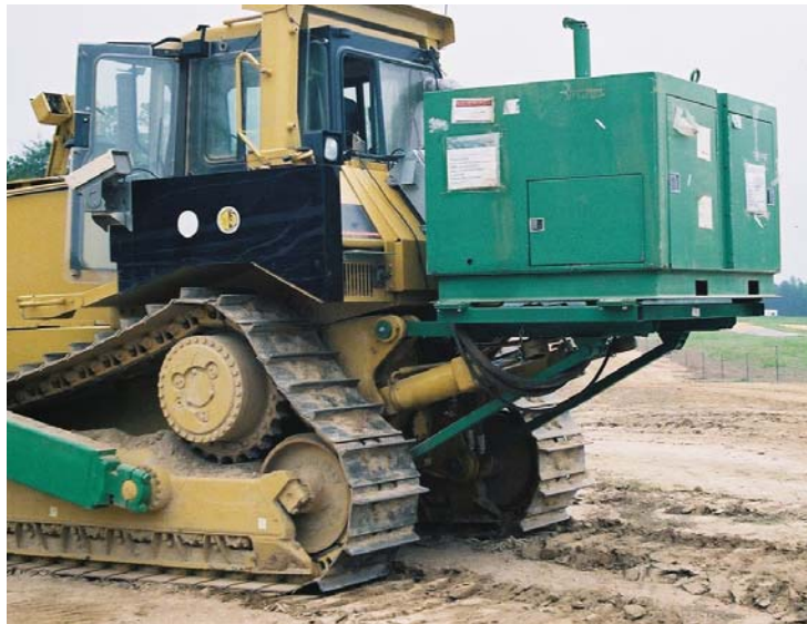
Figure 5 Rear Mounted Hydraulic Power Pack
