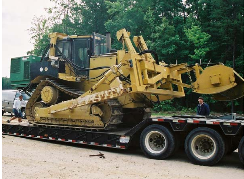
Figure 17 Shredder System and Tractor on Trailer
