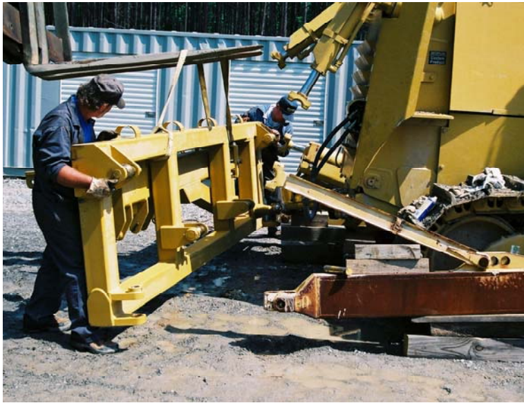
Figure 3 Installation of Mainframe on tractor
