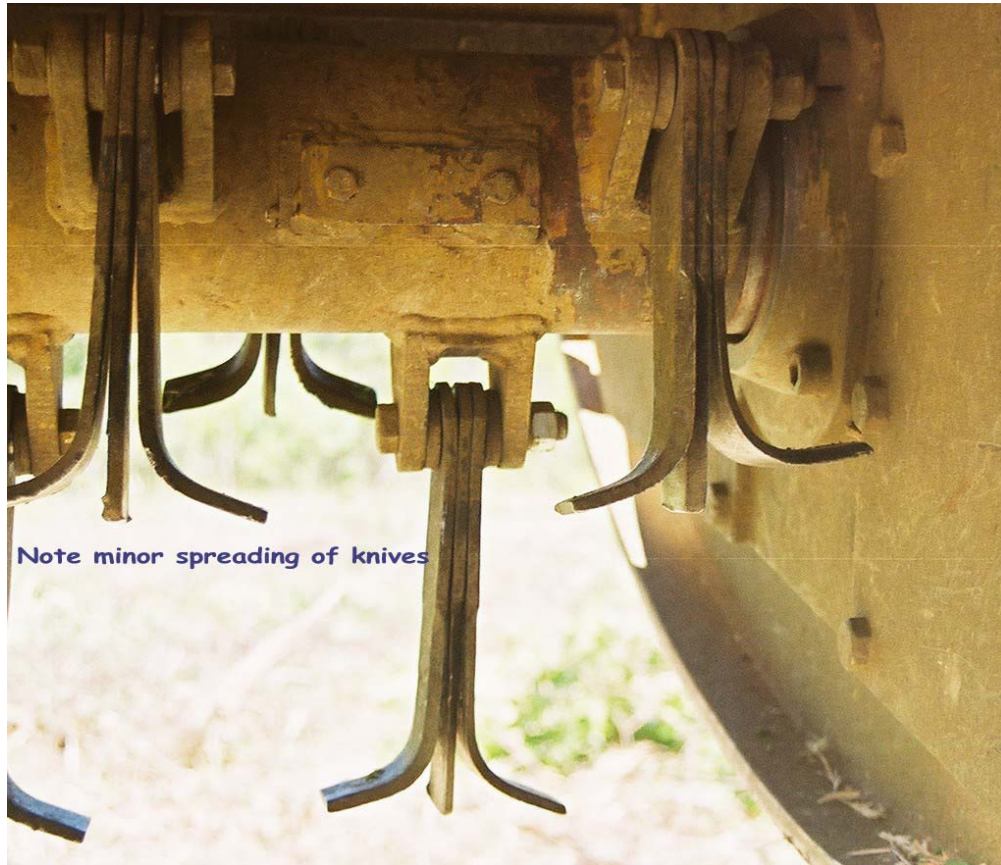
Figure 18 Knives Wear at Test Conclusion
