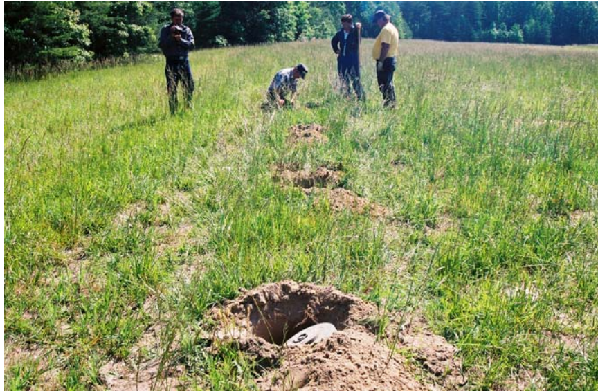
Figure 16 Mine Burial for Sensitivity Test
