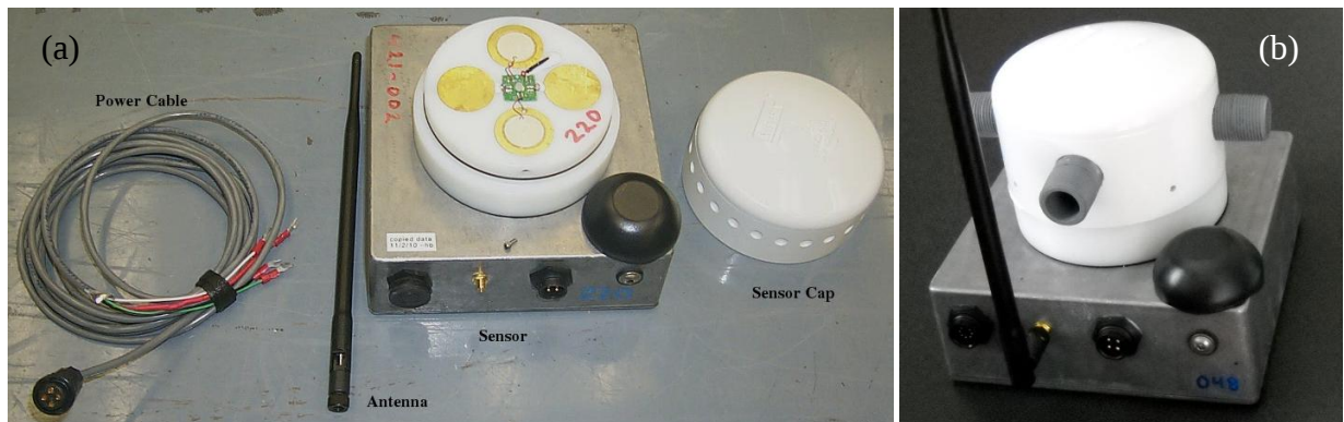
Figure 1. NCPA sensor as it will arrive in the shipping container (a), and assembled using the cap for attaching porous hose (b).
