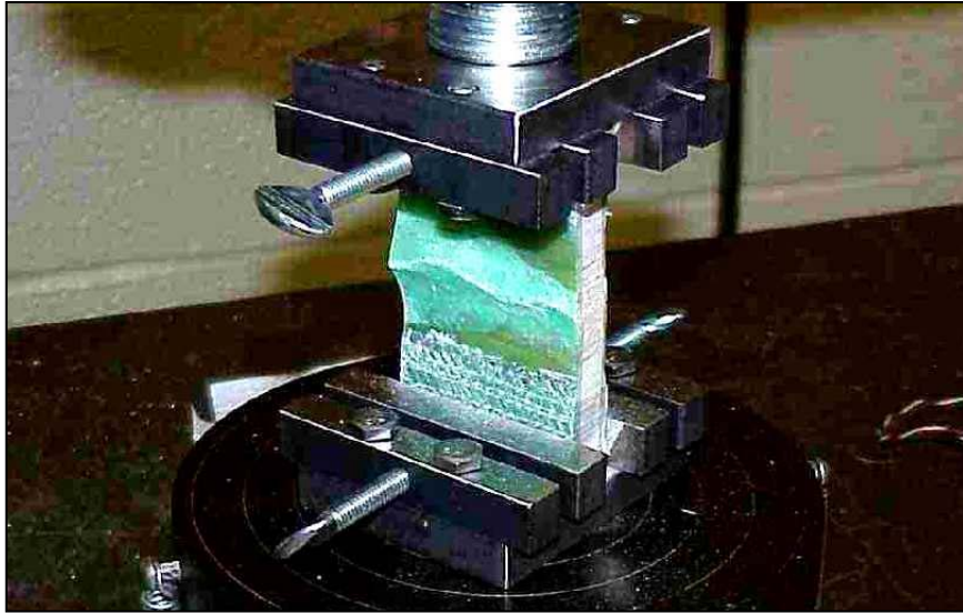
Figure 6-9: Compressive grips with failed specimen
