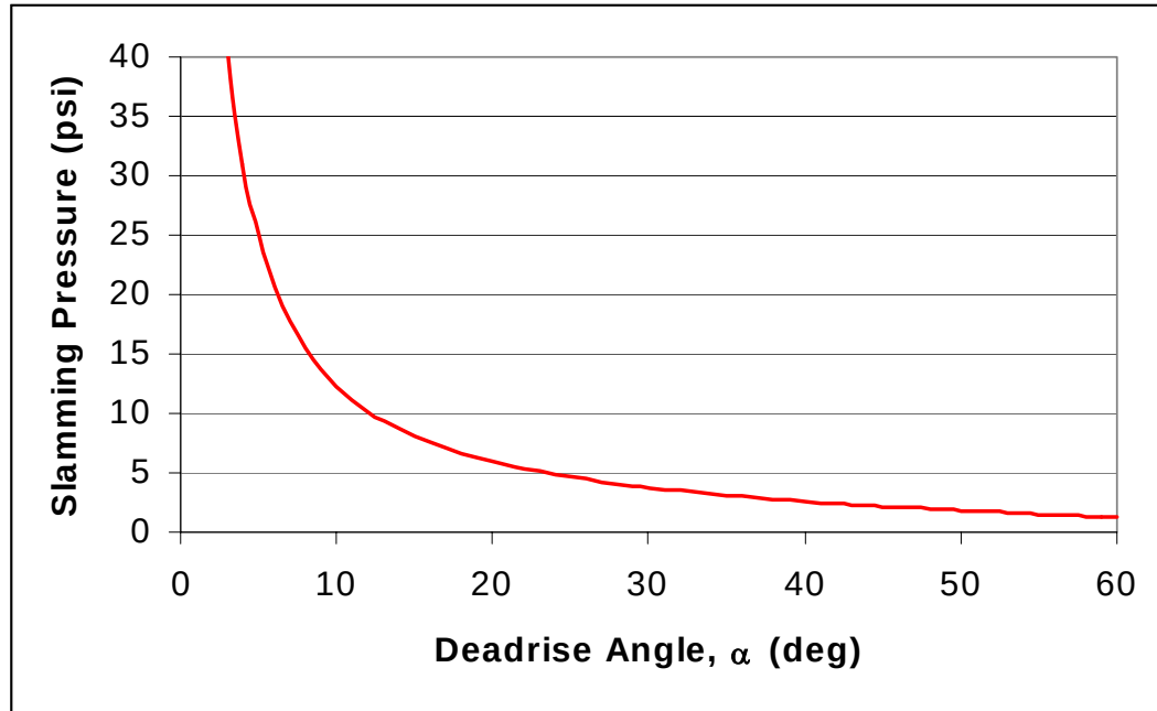
Figure 4-1: Maximum Pressure Due to Slamming ( u=10 fps)
