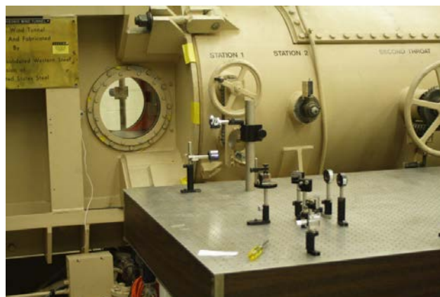
Figure 3. Top: Schematic of the US Air Force Academy Trisonic Wind Tunnel. Bottom: The test section with 0.3-meter-diameter optical windows.
