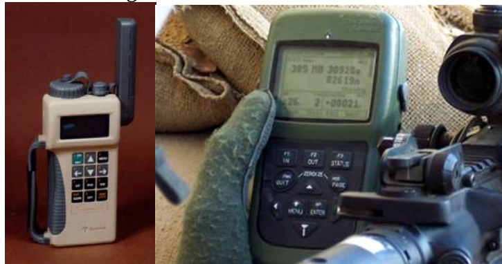
Figure 2-7. Rockwell Collins Precision Lightweight GPS Receiver (PLGR) (left) and Defense Advanced GPS Receiver (DAGR) (right) a later version of the PLGR (Ref. 48, 45)
