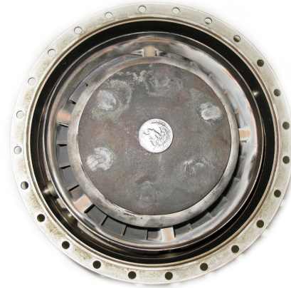
(b) NGV assembly (bottom - heat shield visible)
