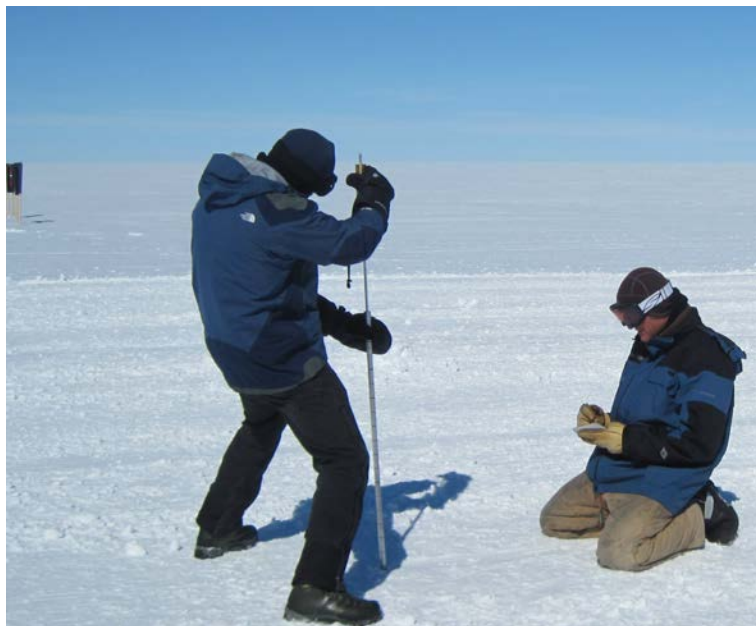
Figure B4. Example of two people taking penetrometer measurements. One is dropping the weight and guiding the penetrometer and the other is taking notes.
