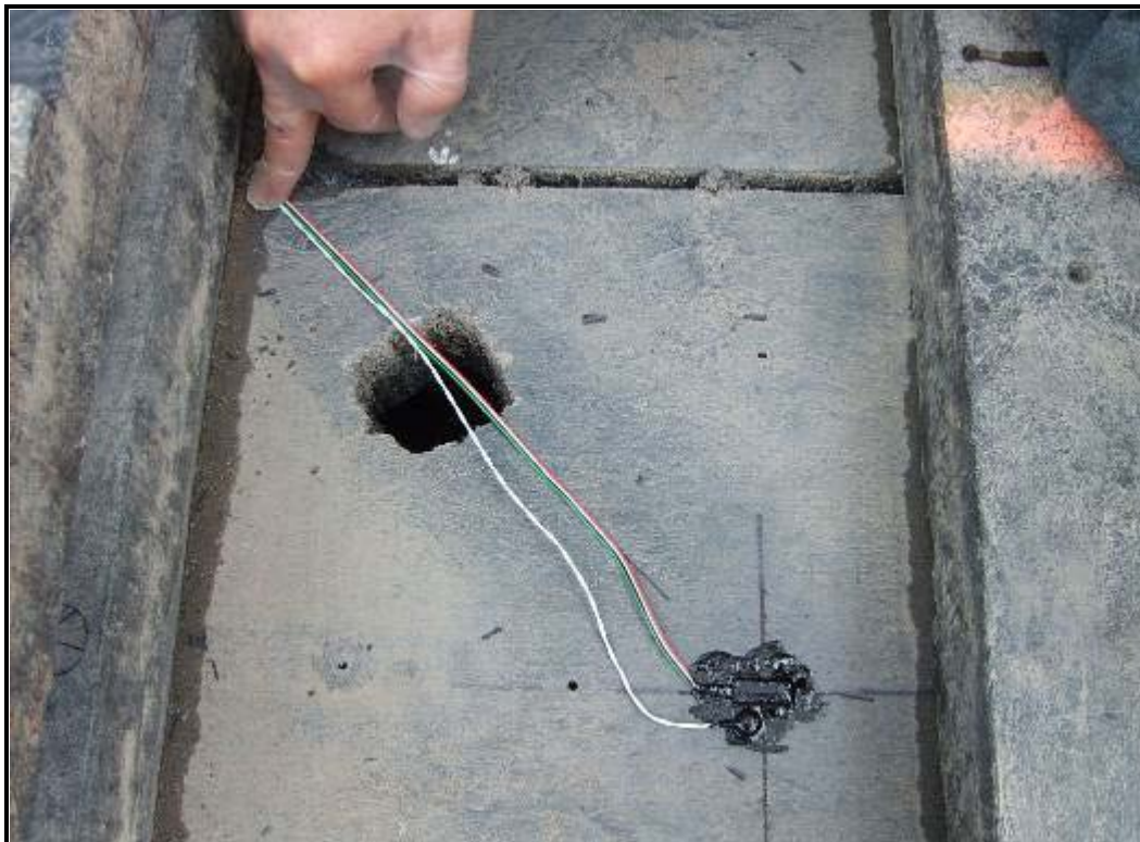
Figure 5. Typical strain gage and surface temperature sensor installation (top of girders at pile cap 3).
