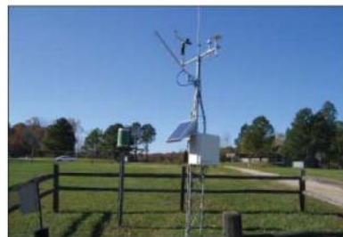
This station for the National Estuarine Research Reserve (NERR) in Virginia transmits data via our GOES satellite transmitter.
