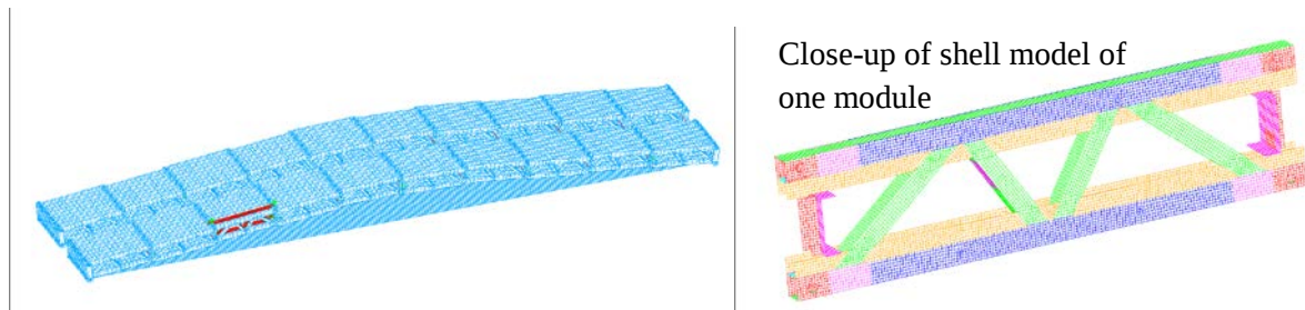
Figure 6. Complete model of entire bridge with all beam elements shown in blue and the spliced-in detailed module shell model in red.
