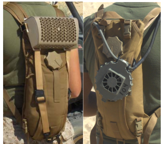
Figure 1: Prototype Beverage Chillers. Left: Non-Powered; Right: Battery-Powered
