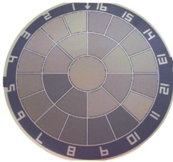
Figure 4. Wafer with 25 different metamaterial configurations.
