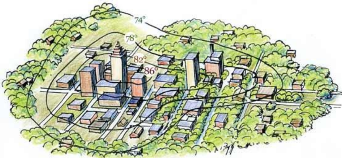
Figure 3. A depiction of the isotherms associated with an urban heat island (Image from the Arbor Day Foundation at arbourday.org ).
