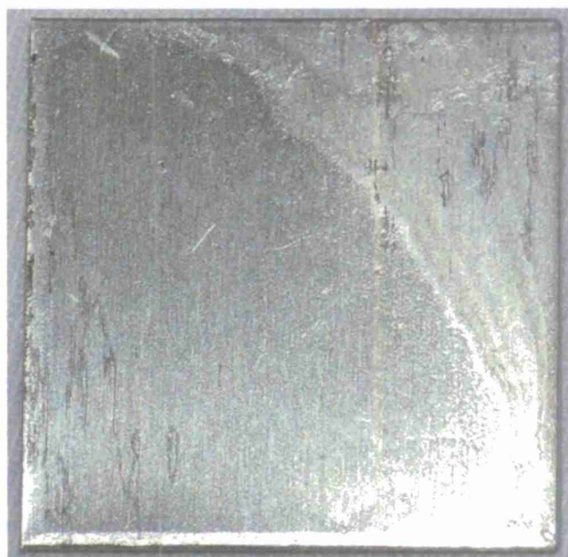
Figure 74. Optical images of AA2024-T351 after 1 week immersion in 50 mM NaCl with Mg shavings and bubbled CO 2 .
