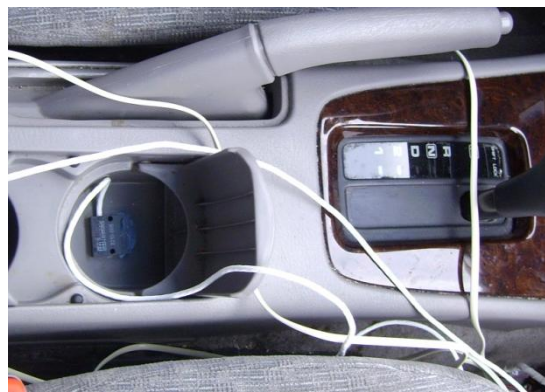
Figure 6: Location of sprung mass accelerometer.
