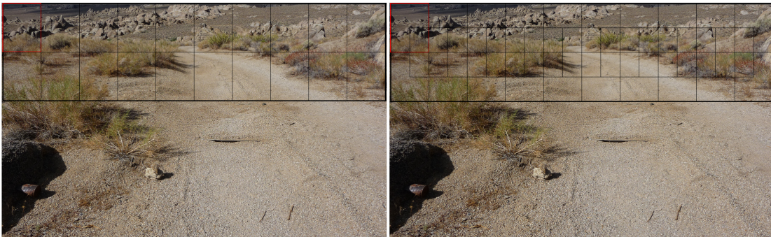
Figure 5.2: Examples of a user-provided training area of the background and the associated break down into smaller rectangles of the same size. In addition, the image on the right shows also the overlapping areas between adjacent rectangles.
