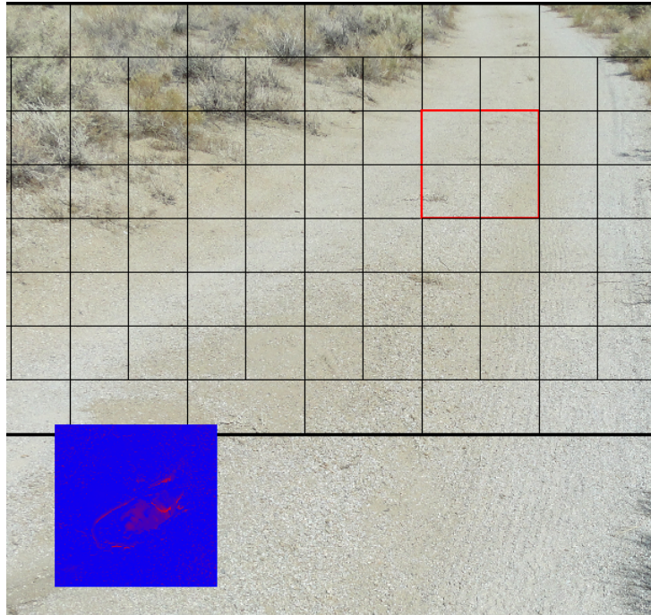
Figure 6.3: The image shows the heat map of an unclassified area. The heat map is generated based on the distance to the referenced background area highlighted in red. This background area is the best matching area for the current unclassified area.
