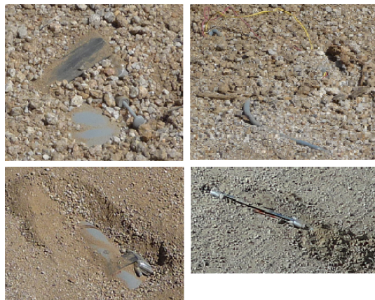
Figure 1.2: Examples of IEDs provided by TRADOC. The IEDs in the second row appear to be closed and monotonically colored. The boundaries are completely visible and in a good contrast to the background. The IEDs shown in the first row are partially hidden, so they do not appear as one closed surface.
