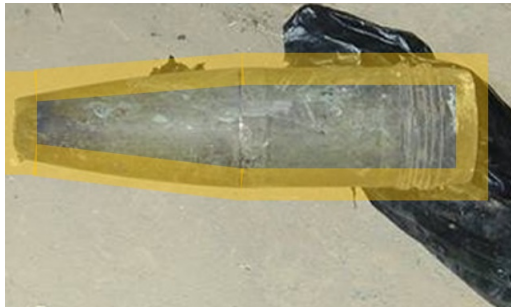
Figure 2.7: A fat pen trail encloses the object boundary. Every pixel outside the trail belongs to the background. Every pixel inside the trail belongs to the object. For all pixels covered by the trail, it is not clear to which segment they belong.
