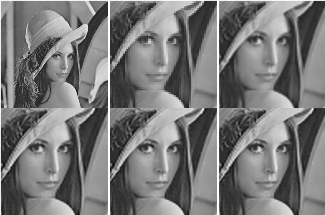
Figure 6: Lena Test. Original image (top left); down-sampled image (top center); Standard bi-cubic reconstruction (top right); First Jacobi iteration of local L^1 -reconstruction (bottom left); Third Jacobi iteration (bottom center); Global L^1 -reconstruction (bottom right);.
