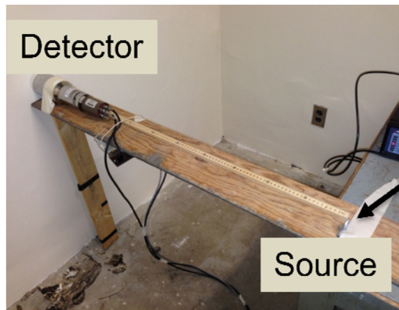
Figure 8: 3x3 NaI detector with pre-amplifier in the experimental configuration
