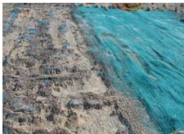
Figure 2. Ultra-violet light degradation of an under-vegetated turf reinforcement mat.
