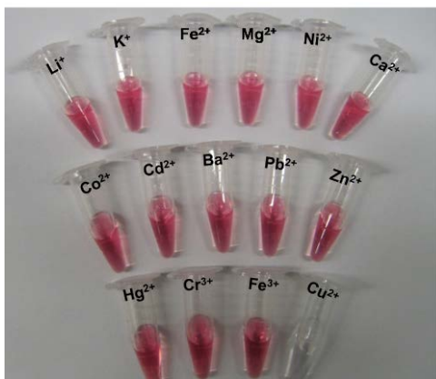
Figure 18. A photograph of the DNA Au NPs at 55 °C in the presence of different metal ions after ligation.
